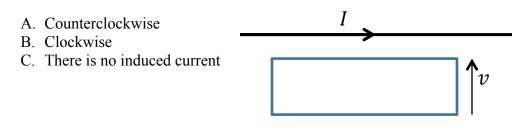
50. A conducting rectangular loop is moving relative to a long, straight current-carrying wire. What is the direction of the induced current in the rectangular loop?
